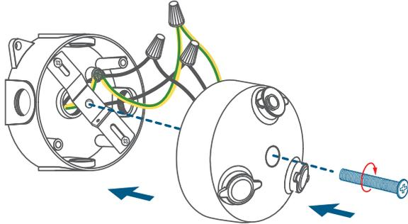
Use the central screw cap to cover the central screw to prevent the central screw from rusting.
