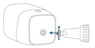
4. Hold and screw the camera to the mounting bracket. Rotate the camera to adjust the view and check it using the live stream, which you can access in the eufy Security app.
