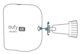
4. Hold and screw the camera to the mounting bracket. Rotate the camera to adjust the view and check it using the live stream, which you can access in the eufy Security app.
