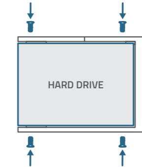
4. Insert and screw the bracket back to S380 HomeBase, then put the top lid back into place.
